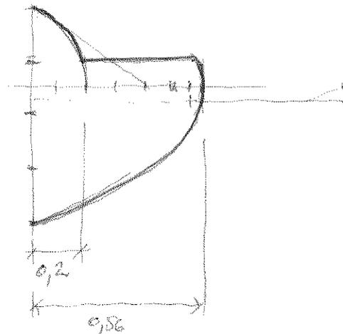
$\dot{\epsilon}_{max} = \frac{2,38 \text{ mKNI}}{12,5 \text{ kN/mm}^2 \times 204 \text{ mm}^2 \cdot \text{m}^2} = 9,68 \times 10^{-3} \text{ m}^{-1} = 3,68 \text{ mrad/m}$      $\delta_{tol} = 10 \text{ mm}$
