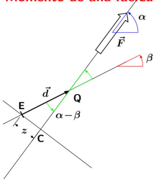
$$\begin{aligned}\vec{M}_E(\vec{F}) &= \vec{F} \times \vec{d} \\ M_E &= F \cdot d \cdot \sin(\alpha - \beta) \\ M_E &= F \cdot z\end{aligned}$$
