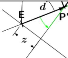
$$\begin{aligned}\vec{M}_E(\vec{F}) &= \vec{F} \times \vec{d} \\ M_E &= F \cdot d \cdot \sin(\alpha - \beta) \\ M_E &= F \cdot z\end{aligned}$$
