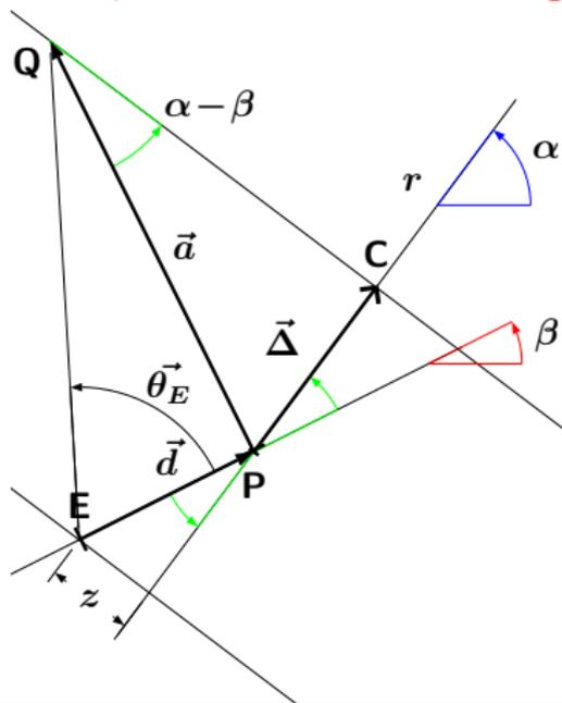
$$\begin{aligned}\vec{a}(\vec{\theta}_E) &= \vec{d} \times \vec{\theta}_E; a = \theta_E \cdot d \\ \Delta &= \theta_E \cdot d \cdot \sin(\alpha - \beta) \\ \Delta &= \theta_E \cdot z\end{aligned}$$
