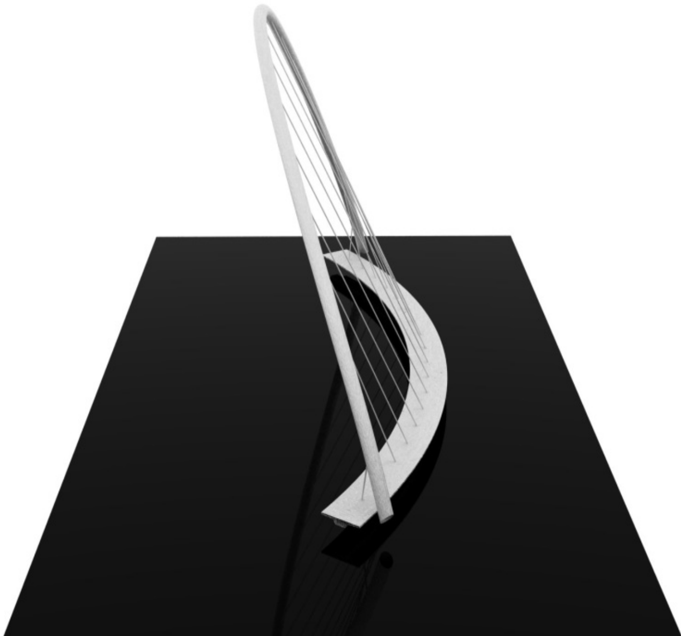
antifunicular arch for bridges with C-shaped deck
